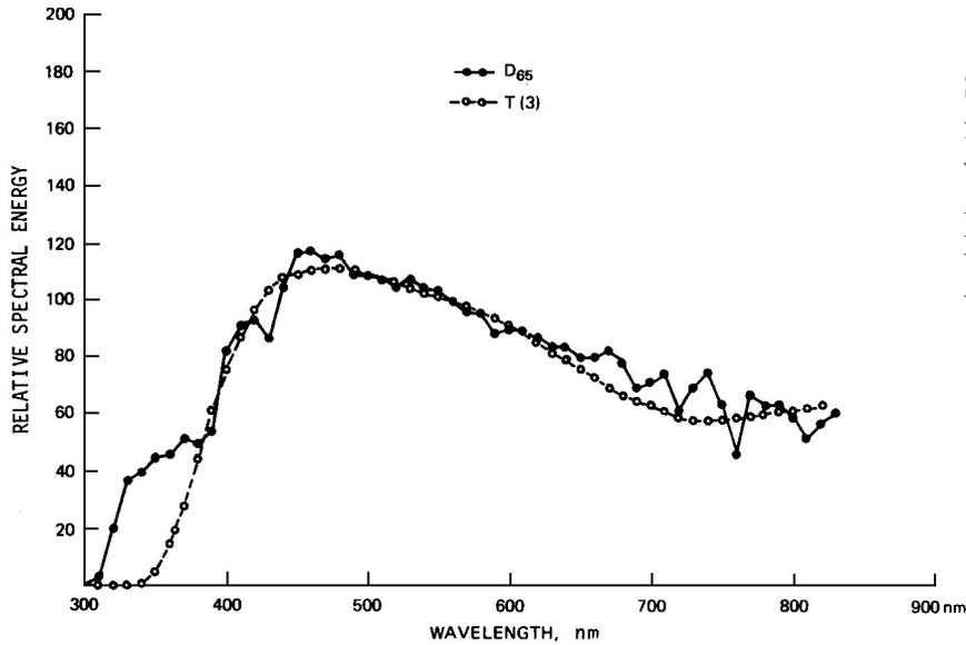
Spectral energy distribution curve for filtered tungsten source compared with illuminant D65 (see legend).
