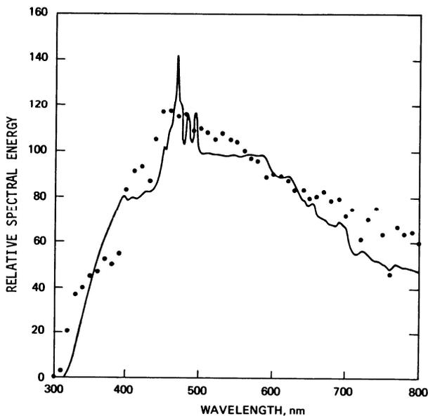
Spectral energy distribution curve for filtered 75-watt xenon lamp (solid line) compared with illuminant D65 (dots).
