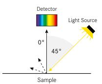
For the blue sample shown beside, a diffuse/8° (also called sphere) geometry instrument will tell you that the sample is the same color on both sides. A 45°/0° (or 0°/45°) geometry instrument will indicate that the halves are different. Which is right? That depends on your need.
