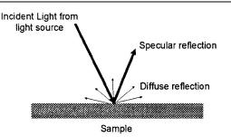
Sphere instruments used in the reflectance specular included mode minimize the effect of differences in gloss, texture, and directionality. For example, if two equally pigmented samples, one glossy and one matte, were measured on a sphere instrument, the readings would indicate that they are roughly equivalent in pigment color, even if they do not appear to be the same visually.
