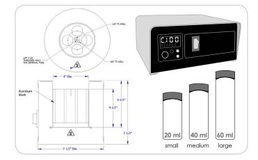
Figure 2. Schematic of the A13-1015-465 Heating Mantle, Temperature Controller and different sizes of glass vials
