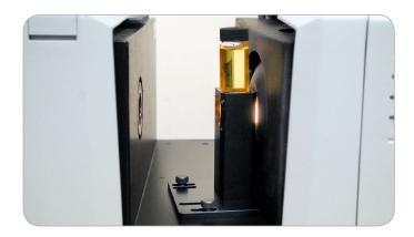
Figure 1. 60 ml Heated Glass Vial (A13-1015-361) in HunterLab Vial Holder (D02-1011-550) for TTRAN Transmission Measurement
