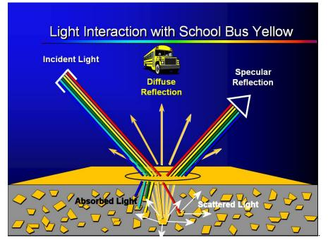
For samples with opacities greater than 75%, the Kubelka-Monk equation (established in 1931) defines a relationship between spectral reflectance (R in %) of the sample and its absorption (K) and scattering (S) characteristics, as follows:
