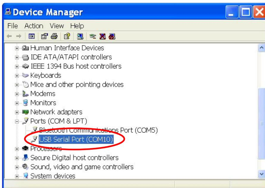
12. Note the COM port number assigned to the USB port you are using. In this example, it is COM10. Once EasyMatch QC is installed and you configure your sensor, you will need to indicate this COM port address as the location for the instrument.
