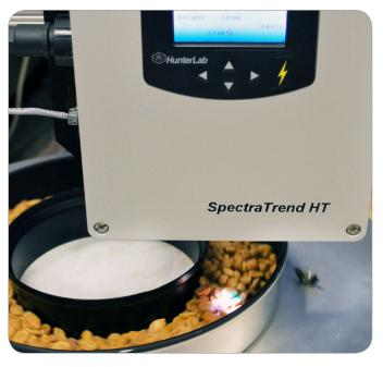
Figure 1. SpectraTrend measuring the color of honey roasted peanuts.
