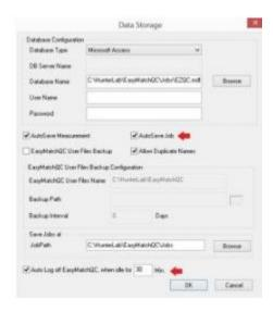
When "AutoSave Job" is checked, the user is prompted for a Job name to save to when the first measurement (Standard or Sample) is taken. From that point on, the Job is "AutoSaved" every tie a new Standard or Sample measurement is taken. This prevents any loss of measurement data by the computer accidentally being shut down.
