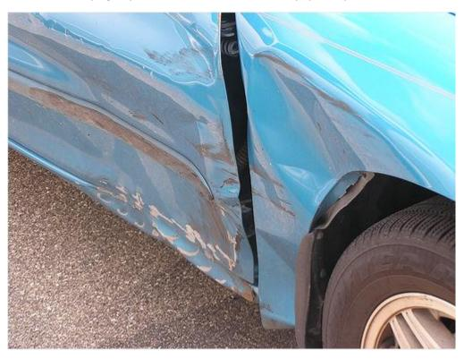
When replacing a damaged quarter panel on a vehicle, the body shop must make sure the pearlescent paint on the new part matches what could be faded paint on the vehicle. Image source: Flickr user heymarchetti
